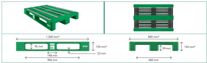
\* The dimensional tolerance is  $\pm$ /- 6 mm for the length and width and  $\pm$ /- 2 mm for the height
